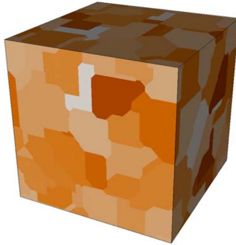
Figure 1: Initial grain structure of the cellular automaton representative volume element with dimensions 256 \times 256 \times 256 \mu\text{m} . The colors are randomly applied to distinguish between grains.
