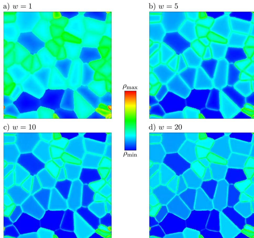
Figure 6: Illustration of the influence of eq. (24) on the distribution of dislocation density in a simulated polycrystal at a strain of 0.1. The parameter  $r_{\min}$  is held constant at  $r_{\min} = 0.5$  while the parameter  $w$  is varied. a)  $w = 1$ , b)  $w = 5$ , c)  $w = 10$  and d)  $w = 20$ . Note the concentration of dislocation density along the grain boundaries.
