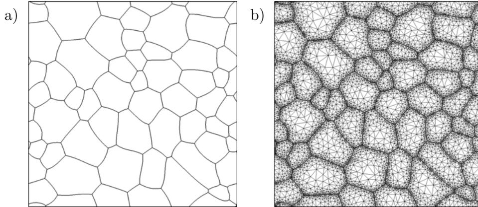
Figure 8: Artificial 2D microstructure used in the simulations. The RVE has outer dimension of  $500 \times 500 \mu\text{m}$  and periodic boundary conditions are applied on the outer boundary. The initial microstructure consists of 52 grains, with an average grain size of  $78 \mu\text{m}$ . a) Grain boundaries, represented by interface segments. b) Mesh discretization from a Delaunay triangulation with approximately 20,000 elements.
